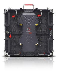
OUTDOOR MIRACKLE P5MM PIXEL PITCH: 5mm Size: 960 x 960 x 80 mm / 37.9"x37.9"x3" Viewing distance: 16ft. High refresh rate: 3840 hz Weight: 60 lbs / 27 Kg Operation power: 100~240V 50-60Hz Max power consumption: 500w/panel Avg. power consumption: 300w/panel
