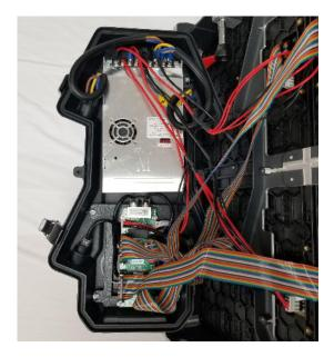
3) Disconnect ribbon cables and power cables from the power supply or receiving card to the panel.
