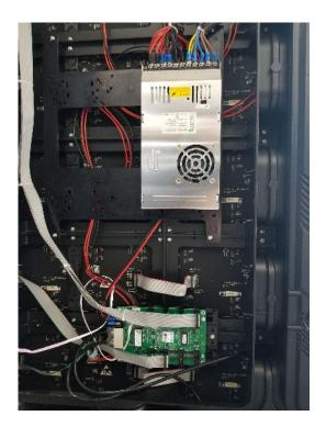
\*We recommend taking a picture of Power Supply, Receiving Card and cable connections before disconnecting any of them. This will help you to not make any mistakes while connecting it back on.
